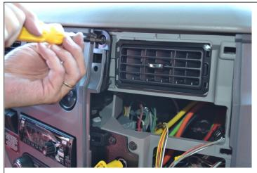
2. Once the panel has been removed, unscrew and remove the upper left dash panel screw. See photo.
