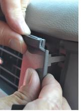
1. Using the included gap opener to get the panel started, gently pull back and take off the dash panel surrounding the upper center dash vent.
