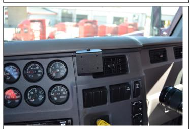
4. Place the dash panel back onto the dash making sure all of the clips are pressed into place. With the shorter machine screw, washers and nut, attach part two of the mount onto part one. position the mount face plate in the direction you would like the face plate to point and securely tighten the machine screw.
