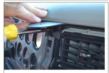
3. Using the included long screw, attach part one of the ProClip mount onto the dash. Place the long screw through the hole in the mount and thread the screw into the dash where the dash screw was removed. Fasten part one of the mount securely onto the dash.
